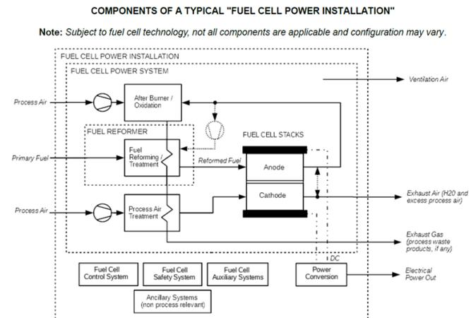
Figure 6. CCC4/WP.3 fuel cell system diagram
