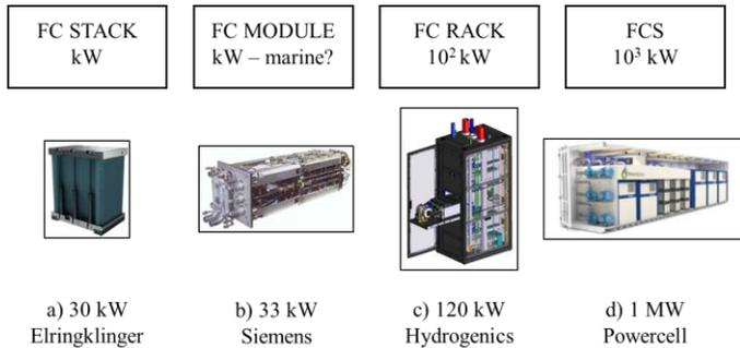
Figure 7. PEMFC scale up scheme
