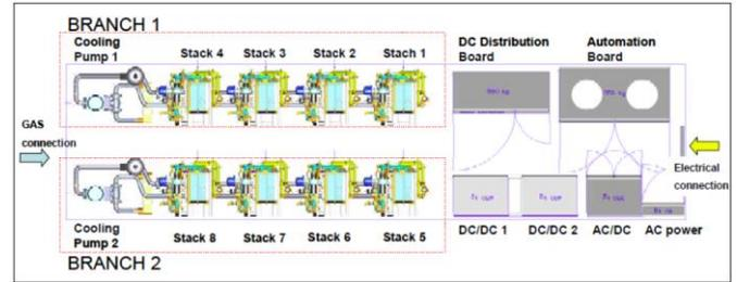
Figure 2. FCS test rig configuration
